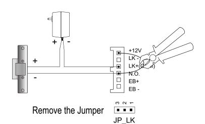
set to Normally Closed on the Unlock Relay mode
