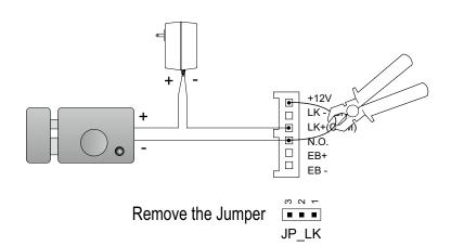
set to Normally Open on the Unlock Relay mode (default)
